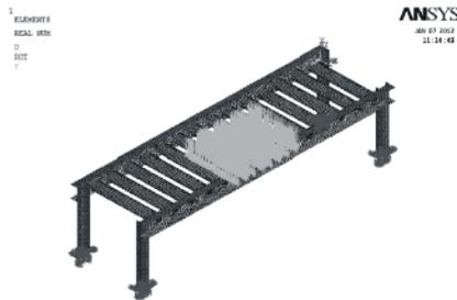
Fig. 6. A static load of 3500 N (approx 350 kg) is applied on the 4 rollers at the centre, as the deflection will be maximum, when the load is applied at the centre.
