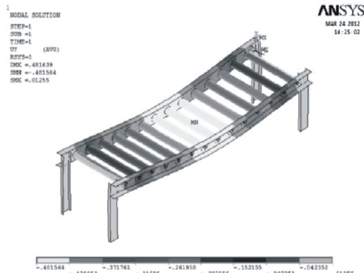
Fig. 10. Linear Static Analysis of Optimized design: Deflection plot.
