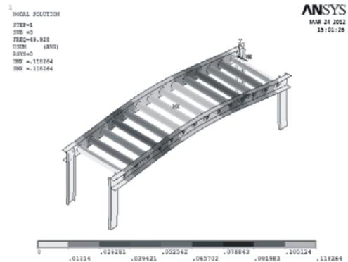
Fig. 12. Critical Mode Shape of Optimized design.
